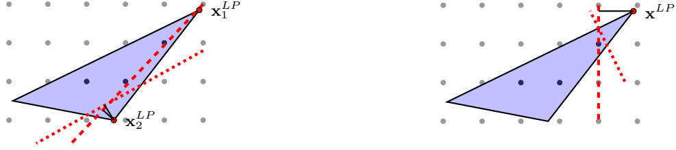
(a) The dashed cut removes the entire optimal face, and thereby is likely preferable. Efficacy however scores the cut higher (black lines). Analytic, minimum, and average efficacy prefer the dashed cut. (b) The projection from \mathbf{x}^{LP} onto the dashed cut is LP-infeasible, limiting its usefulness as a measure. The dotted cut is dominated but would still be selected by efficacy.
