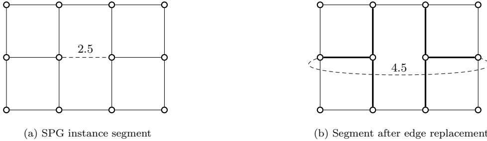
Figure 5: Segment of a Steiner tree instance (showing only non-terminals). All edges except for the dashed ones have unit weight. The dashed edge in (5a) has been replaced in (5b). All edges that are in conflict with the replacement edge in (5b) are drawn in bold.
