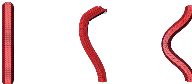
Figure 2: Example 2. Left: linear elastomechanics. Center: geometric nonlinearity with linear St. Venant-Kirchhoff material. Right: geometric nonlinearity with OGDEN material ( d = 10^5 ).
