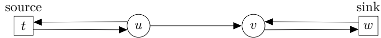
Figure 3: All arcs a in this network are shortcuts with \underline{q}_a = 0 and \bar{q}_a = \infty . With exception of (u, v) they do not carry information and can be contracted. However, (u, v) may not be contracted as it carries the information that no flow is permitted from w to t , but only in the opposite direction.
