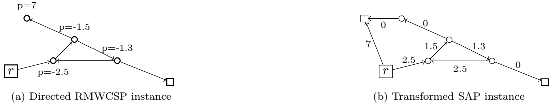
Figure 5: Illustration of a directed RMWCSP instance with root r (left) and the equivalent SAP obtained by Transformation 2 (right). Terminals are drawn as squares.
