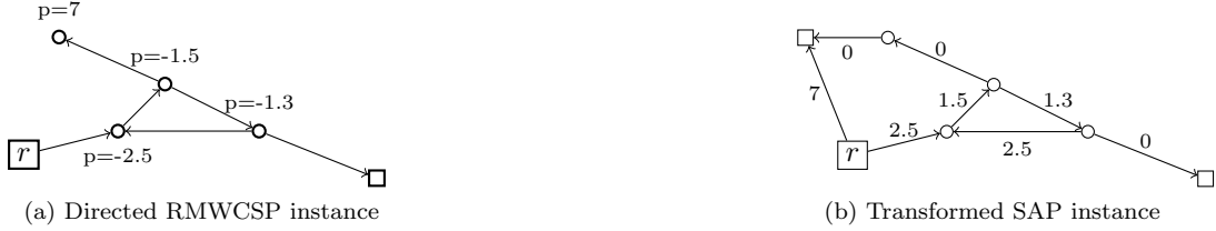
Figure 3: Illustration of a directed RMWCSP instance with root r (left) and the equivalent SAP obtained by Transformation 2 (right). Terminals are drawn as squares.
