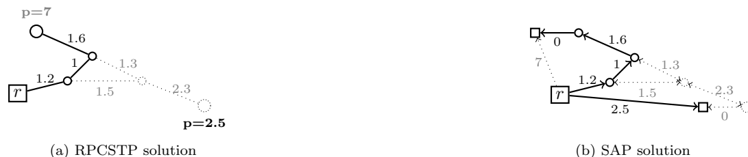
Figure 4: Illustration of a solution to the RPCSTP instance of Figure 3 (left) and an equivalent solution to the corresponding SAP (right).
