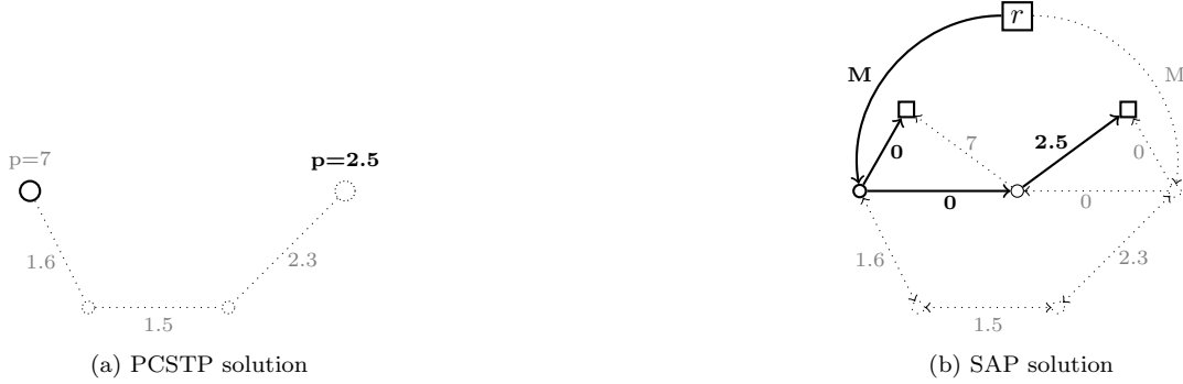
Figure 4: Illustration of the (single-vertex) optimal solution to the PCSTP instance depicted in Figure 3 (left) and the equivalent solution to the corresponding SAP (right).
