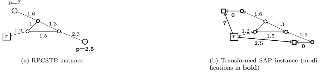
Figure 1: Illustration of an RPCSTP instance with root r (left) and the equivalent SAP obtained by Transformation 1 (right). Terminals are drawn as squares and Steiner vertices as circles (with those of positive weight enlarged).
