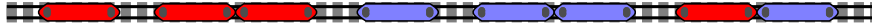
Fig. 1 Possible vehicle configurations composed of two fleets, i.e., a red fleet and a blue fleet.
