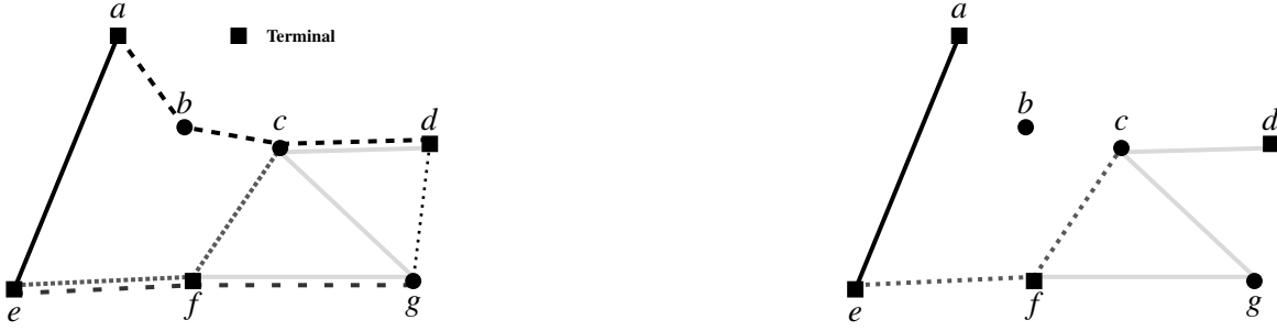
Figure 1: Example of a Steiner connectivity problem. Left: A graph with four terminal nodes ( T = \{a, d, e, f\} ) and six paths ( \mathcal{P} = \{p_1 = (ab, bc, cd), p_2 = (ef, fg), p_3 = (ae), p_4 = (ef, fc), p_5 = (gd), p_6 = (fg, gc, cd)\} ). Right: A feasible solution with three paths ( \mathcal{P}' = \{p_3, p_4, p_6\} ).
