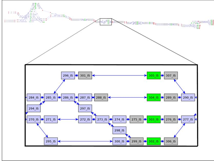
**Figure 5:** Microscopic network of the Simplon and detailed representation of station Iselle as given by OpenTrack
