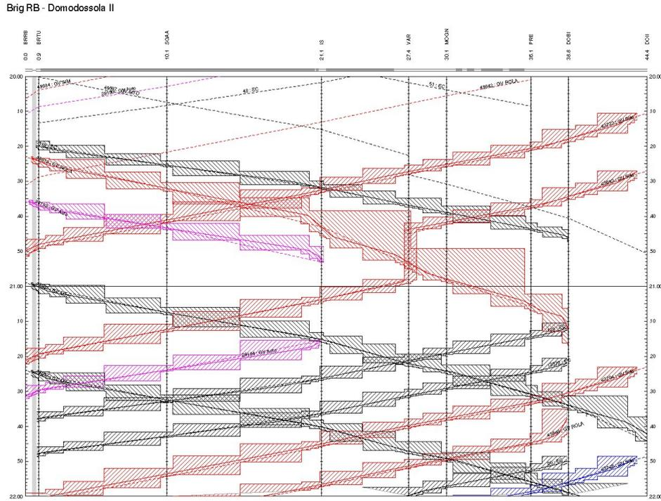
**Figure 12:** Traffic diagram in OpenTrack with block occupation for request 24h-tp-as
