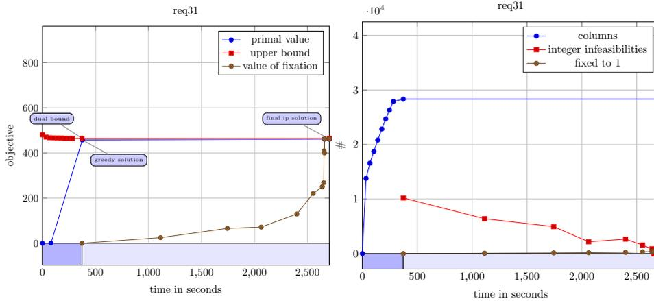
**Figure 7:** Solving a track allocation problem with TS-OPT; dual (LP) and primal (IP) stage.
