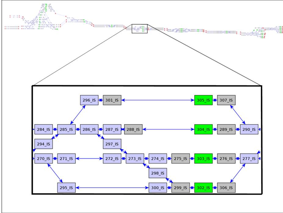
**Figure 10:** Micro graph representation of Simplon and detailed representation of station Iselle given by OpenTrack.
