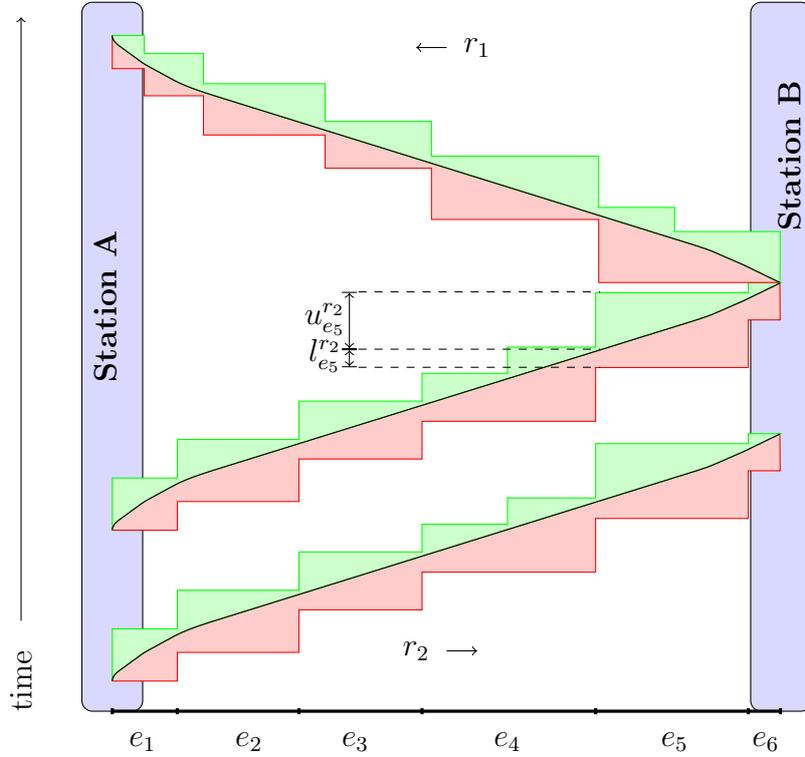
**Figure 6:** Blocking time diagrams for three trains on two routes using 6 blocks. In the lower part of the diagram two subsequent trains on route  $r_2$  and at the top one train on the opposite directed route  $r_1$  are shown.
