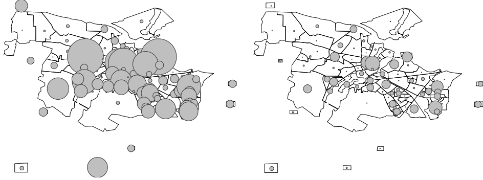
Figure 5: Results for optimizing the current fare system with single/monthly ticket using model MAX-R. Potsdam is subdivided into 86 districts; the size of the circle in each district is proportional to the number of passengers which arrive at the district by car ( Left ) and public transport ( Right ).
