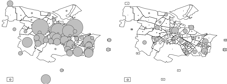
Figure 4: Results for optimizing the current fare system with single/monthly ticket using model MAX-R. Potsdam is subdivided into 86 districts; the size of the circle in each district is proportional to the number of passengers which arrive at the district by car ( Left ) and public transport ( Right ).
