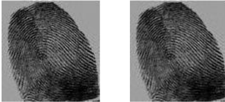
Figure 4: Deblurring results obtained using the models (4.4) left and (4.2) right, with \phi(\xi) = \sqrt{\epsilon + |\xi|^2} (total variation minimization with regularization).
