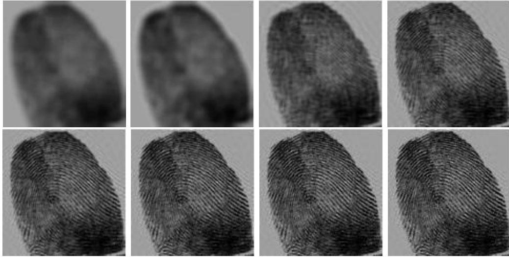
Figure 3: Top left to bottom right: blurred image, several iterates using (4.4): 1st, 100th, 500th, 1000th, 2000th, 3000th, 4000th.
