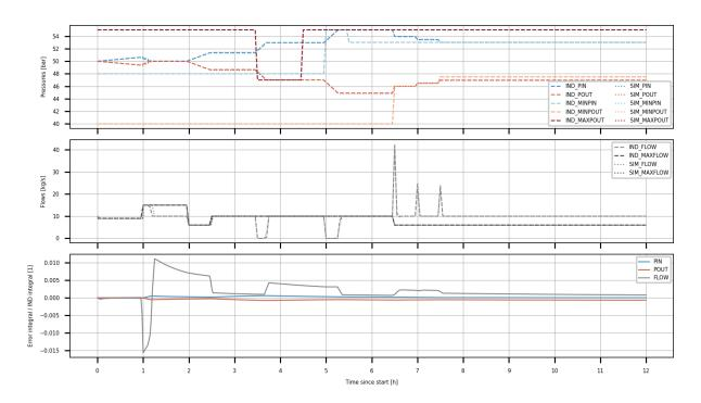
Figure 4: Comparison of the simulated solution (SIM) with the reference simulation from the industry simulator (IND) for the first scenario with predefined target values based on Table 3. The pictures show the left and right pressure values and target values of the regulator, the flow values and target values, and the difference of both solutions in the three quantities integrated over time and normalized by the quantity integral of the IND values.
