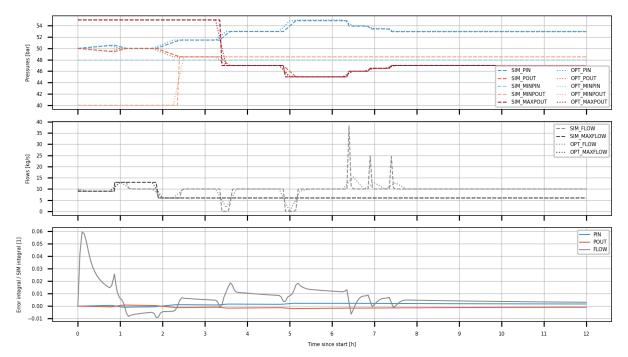
Figure 9: Comparison of the optimized solution (OPT) with the reference simulated solution (SIM) for the second scenario with optimized target values, see Table 4. The pictures show the left and right pressure values and target values of the regulator, the flow values and target values, and the difference of both solutions in the three quantities integrated over time and normalized by the quantity integral of the SIM values.
