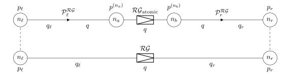
Figure 1: Depiction of the hidden sub-network structure (above in the picture) behind a regulator or sometimes control valve  $\mathcal{RG}$  (below in the picture), including an atomic regulator  $\mathcal{RG}_{\text{atomic}}$  as well as two internal pipes  $\mathcal{P}_{\ell}^{\mathcal{RG}}$  and  $\mathcal{P}_{r}^{\mathcal{RG}}$ .
