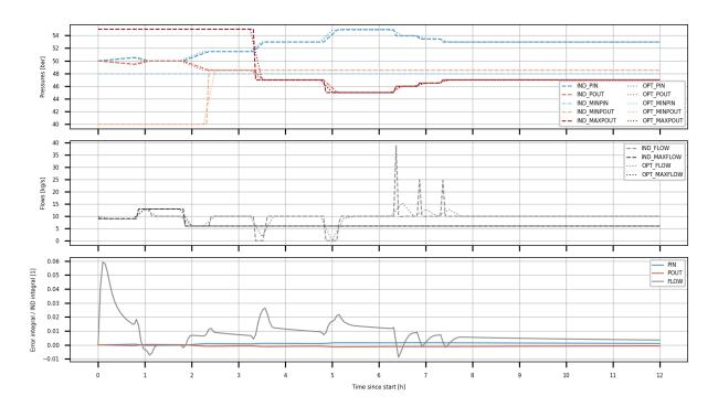
Figure 8: Comparison of the optimized solution (OPT) with the reference simulation from the industry simulator (IND) for the second scenario with optimized target values, see Table 4. The pictures show the left and right pressure values and target values of the regulator, the flow values and target values, and the difference of both solutions in the three quantities integrated over time and normalized by the quantity integral of the IND values.
