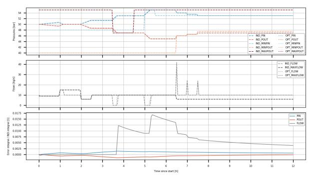
Figure 5: Comparison of the optimized solution (OPT) with the reference simulation from the industry simulator (IND) for the first scenario with predefined target values based on Table 3. The pictures show the left and right pressure values and target values of the regulator, the flow values and target values, and the difference of both solutions in the three quantities integrated over time and normalized by the quantity integral of the IND values.
