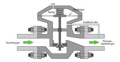
Figure 2: Visualization of a regulator controlling the right pressure; picture created by [Kuphaldt, 2019], published under CC BY  $4.0^2$
