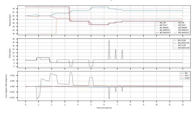
Figure 7: Comparison of the simulation (SIM) with the reference simulation from the industry simulator (IND) for the second scenario with optimized target values, see Table 4. The pictures show the left and right pressure values and target values of the regulator, the flow values and target values, and the difference of both solutions in the three quantities integrated over time and normalized by the quantity integral of the IND values.
