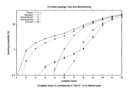
FIGURE 5. Blocking probability of the algorithms on the 14-nodes network with low cost dimensioning
