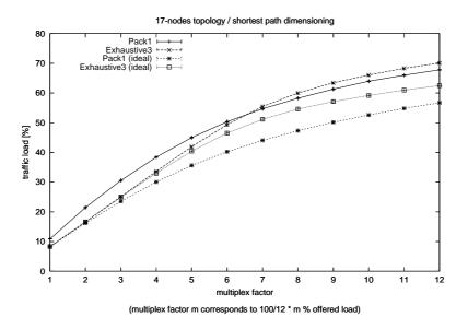
FIGURE 10. Ideal network loads for two algorithms on the 17-nodes network with shortest path dimensioning
