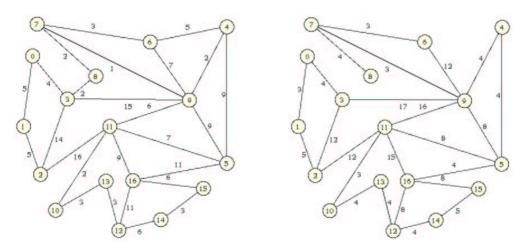
FIGURE 11. The 17-nodes network with shortest path and with low cost dimensioning
