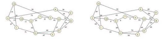
FIGURE 12. The 14-nodes network with shortest path and with low cost dimensioning
