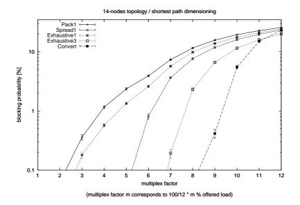
FIGURE 4. Blocking probability of the algorithms on the 14-nodes network with shortest-path dimensioning
