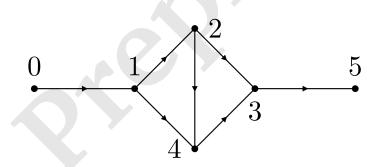
Fig. 3 gas\_diamond - gas transportation network with 6 nodes and 7 arcs.
