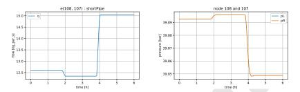
**Fig. 12** gas\_N138\_A139 – pipe node\_72\_ld42 (connecting the innode (name: node\_72, idx: 108) with sink node (name: node\_ld42, idx: 107): flow and pressure curves
