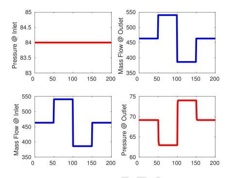
Fig. 2 Input-Output behavior for the pipeline benchmark. Upper left: Pressure at inlet, upper right: mass flow at outlet, lower left: mass flow at inlet, lower right: pressure at outlet.
