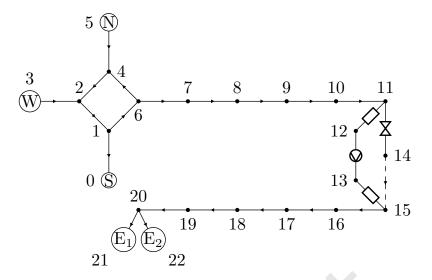
**Fig. 6** gas\_N23\_A24 – gas transportation network with 23 nodes and 24 arcs. The dashed line represents a short pipe. The node enumeration corresponds to that defined in the benchmark function (for viewing results).
