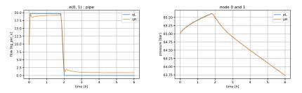
**Fig. 11** gas\_N138\_A139 – pipe p\_brl (connecting the source node (name: node\_l, idx: 0) with innode (name: node\_2, idx: 1): flow and pressure curves
