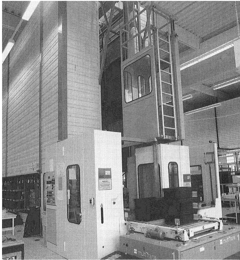
Figure 2.2.3 AGV at the automatic storage system
