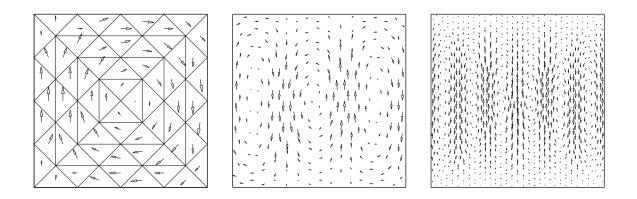
Figure 5: Grid structure and electric field for  $\omega = 1.5\pi$  (left hand side), field for  $\omega = 3\pi$  (center), and field for  $\omega = 6\pi$  in experiment 1.
