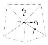
Figure 3: Triangulation with global Cartesian coordinate axes  $e_1$  and  $e_2$  at vertex m.
