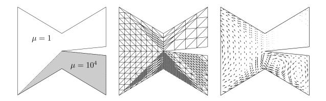
Figure 6: Values for  $\mu$  on the domain (left hand side), adaptively refined grid (center), and electric field in experiment 2.
