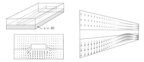
Figure 7: Tapered microstrip line on a dielectric substrate with  $\epsilon = 10$  (top left). Electric field on a cross section (bottom left) and on the central plane along the conductor (experiment 3).
