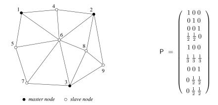
Figure 1: Distribution of master and slave nodes on a two-dimensional grid and the resulting prolongation matrix *P*. For practical reasons, the lowest numbers have been assigned to the master nodes, which will be retained on the coarse grid.
