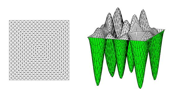
Figure 4: Exp. 3: Grid and solution for the Helmholtz equation.
