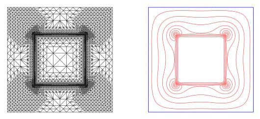
Figure 3: Adaptively refined grid of Exp. 2 (left) and contour lines of the vector potential  $A_z$ .
