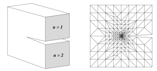
Figure 5: 3D-region with crack (Exp. 4): structure with applied boundary conditions (left) and cross-section of an adaptively refined grid.
