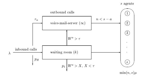
Figure 4.1. Call center with impatient inbound calls and overflow into a voice-mail-server (VMS) occurring directly at the arrival (state dependent on the number n of calls being in service or in the waiting room) or after a deterministic maximal waiting time  $\tau$ .
