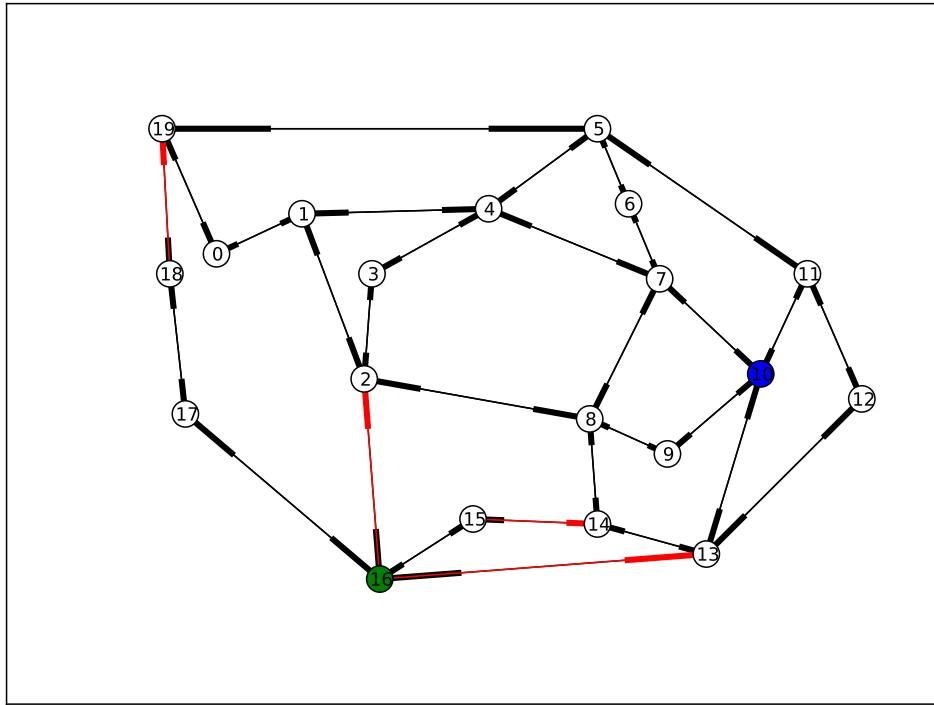
On this graph, the source in blue, the sink in green, and the edges defining the cut are marked in red.
