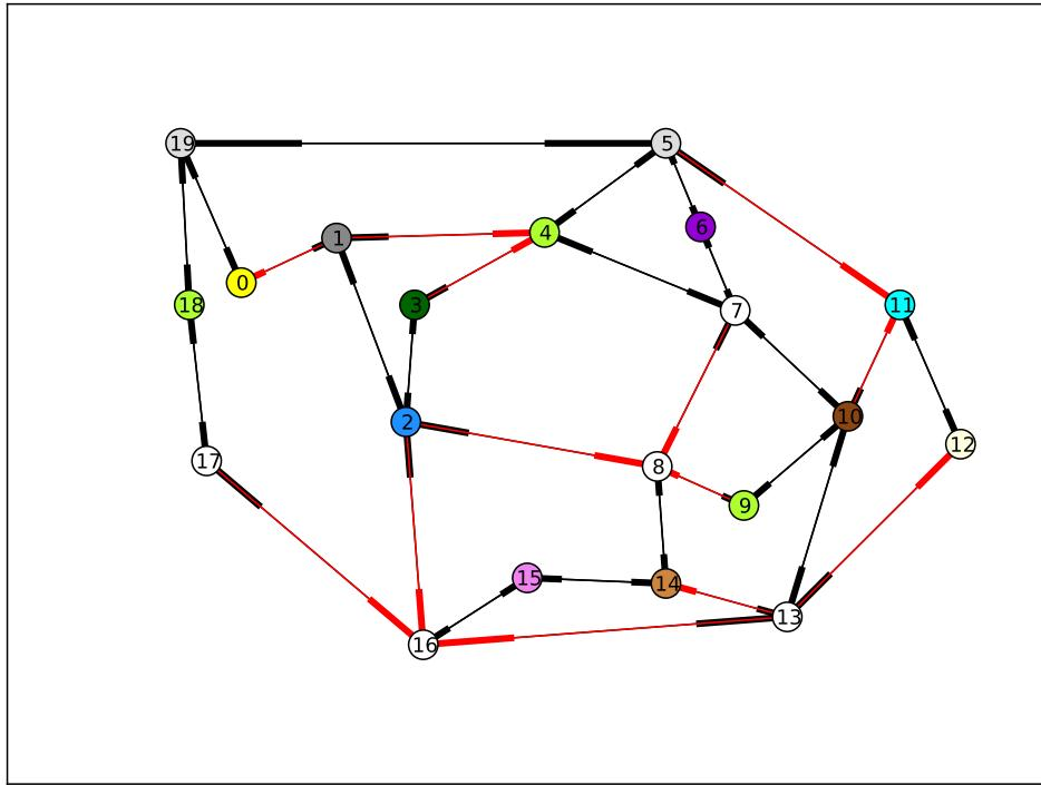
On this graph, the pairs of terminal nodes are denoted by dark and light colors of the same shade (e.g. dark vs. light green for the pairs (3,4),(3,9), and (3,18)), and the edges defining the cut are marked in red.
