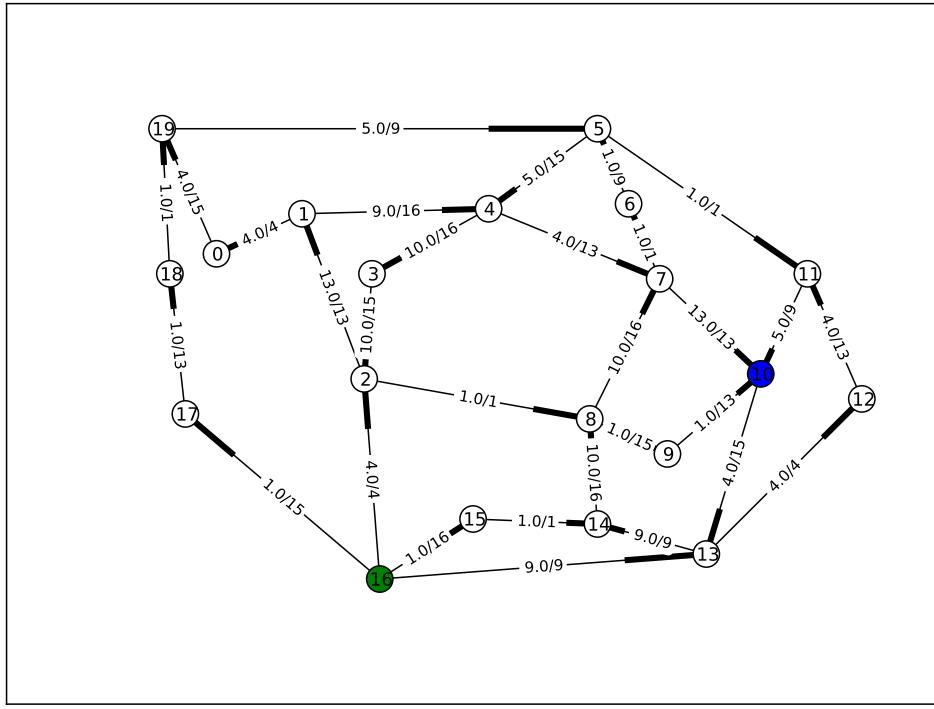
The graph shows the source in blue, the sink in green, and the value of the flow together with the capacity on each edge.
