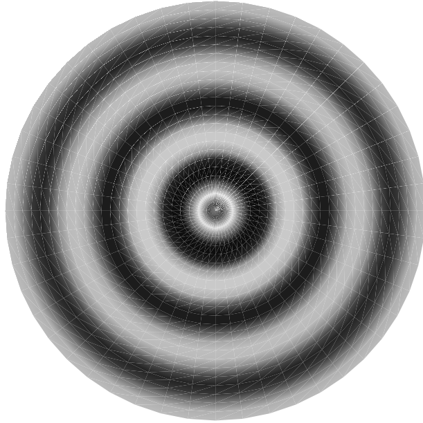
Figure 3: Eigenfunction for n = 0 , \lambda = 0.6680 , and R = 24 .
