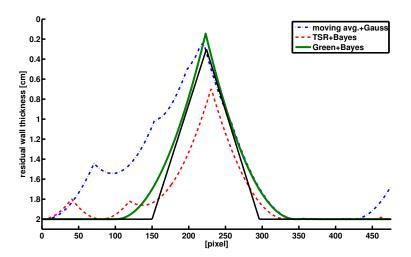
Figure 8: Experimental data: Reconstruction for the 120°-triangle for different preprocessing techniques.
