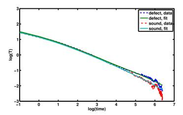
Figure 7: Experimental data: Fitted surface temperature above defect and sound area (detail).
