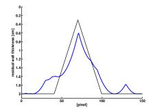
Figure 5: Simulation data. Reconstruction using the Envelope Algorithm [6] for the  $a=120^{\circ}$ -triangle and  $\sigma_2=1K$  with Green (left) and moving average (right), both applied before using Gauss filter in space with  $\sigma^2=0.5$ . As a reference temperature for contrast computation,  $\hat{T}(0,t)$  was used. Thresholds for the thermal contrast were 0.075.
