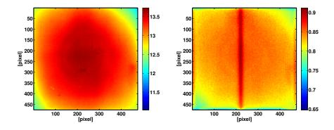
Figure 6: Experimental data: Surface temperature directly (left) and 22s (right) after heating.
