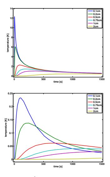
Figure 2: Top: Solutions  $\hat{T}(z_i,t)$  to Eq. (1) for  $T_0 = T_{\rm ext} = 0$  and different depths  $z_i$ . Bottom: Front surface temperature  $T_{L_i}(0,t)$  for Eq. (2) for rear in different depths  $L_i$ .
