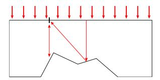
Figure 1: The temperature evolution on the surface can be modeled as a superposition of contributions with different path lengths.
