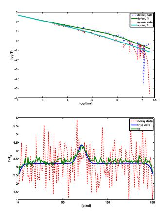
Figure 4: Simulation data. Top: Fitted surface temperature above defect and sound area for the  $a=120^{\circ}$ -triangle and  $\sigma_1=0.2K$  (detail). Bottom: Temperature over a cross section in space at t=87.5s for  $\sigma_2=1K$ .
