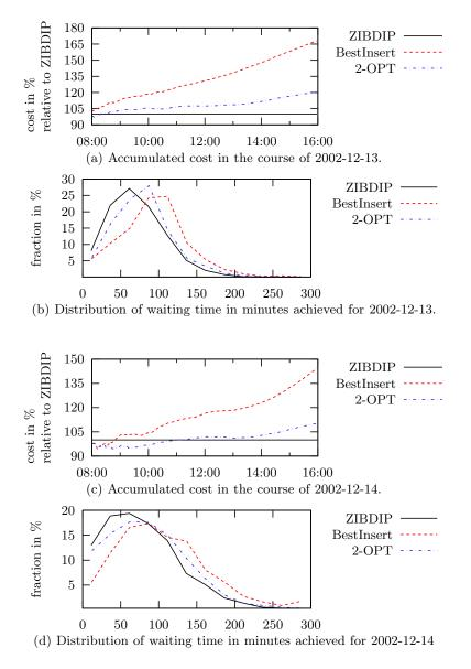
Fig. 5. Comparison of ZIBDIP to two heuristics on two high load days [9].
