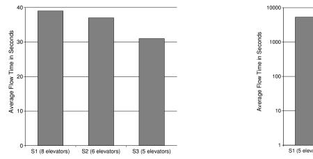
(a) Number of elevators needed to serve a 16 floor system with average flow time at most 40 seconds for FIFO (S1), NN (S2), and REOPT (S3)
