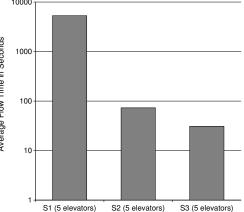
(b) Average flow time achieved by FIFO (S1), NN (S2), and REOPT (S3) on a 5 elevator 16 floor system. Note that the y-axis is logarithmic.
