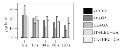
Fig. 3. Comparison of ZIBDIP with several variants of genetic algorithms. Depicted is the deviation from the optimal cost in percent after a given computation time. The data is taken from [13].
