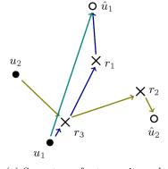
(a) Some tours for two units and three requests  $r_1, r_2, r_3$ .  $u_1$  and  $u_2$  indicate the current positions of both units and  $\hat{u}_1$  and  $\hat{u}_2$  their home positions.
