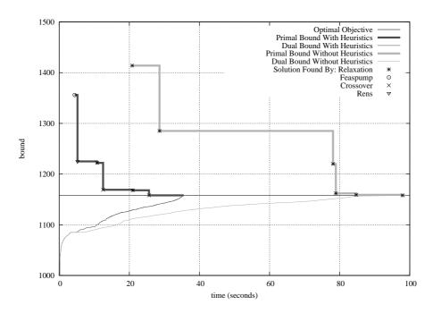
Figure 1: Instance aflow30a: developing of primal and dual bound if SCIP runs with (dark) and without any heuristics (light)
