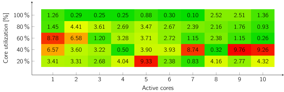
Figure 4.8: CPU power model relative error percentage.
