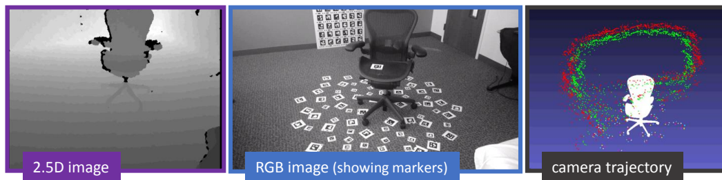
Fig. 3.11: Real data acquisition and processing. From left to right: sample real depth data ; sample RGB data with markers ; recovered trajectory (poses) for each samples (for Chair C ).
