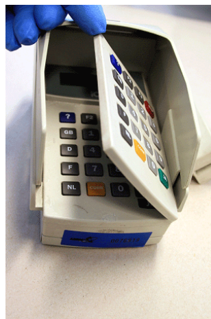
Figure 1.3: Cardblocker PIN reader terminal topper
