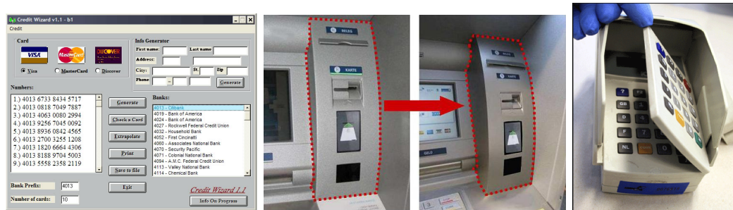
Figure 1.1: (Left) Credit-card number generation tool: Credit Wizard, (Middle) Skimming devices integrated into a fake front panel of an ATM, (Right) Fake PIN-pad on a POS terminal. 6
