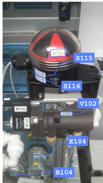
Figure 1: Close view of (parts of) a water management plant model with physical tagging
