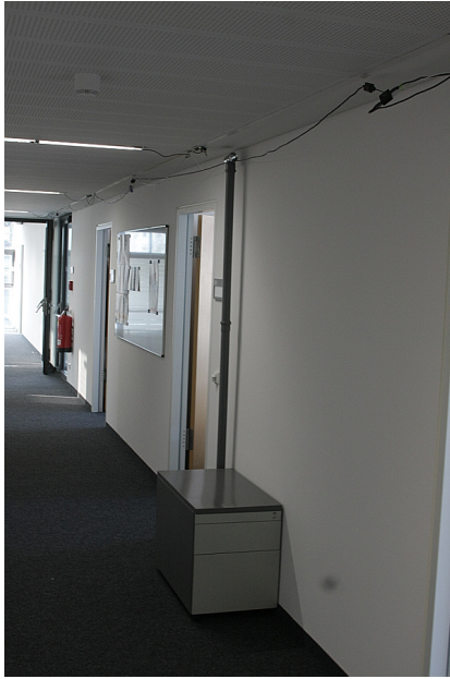
(a) Corridor: 15 sensors, 48 days, height 2.40m, and area 124m 2
