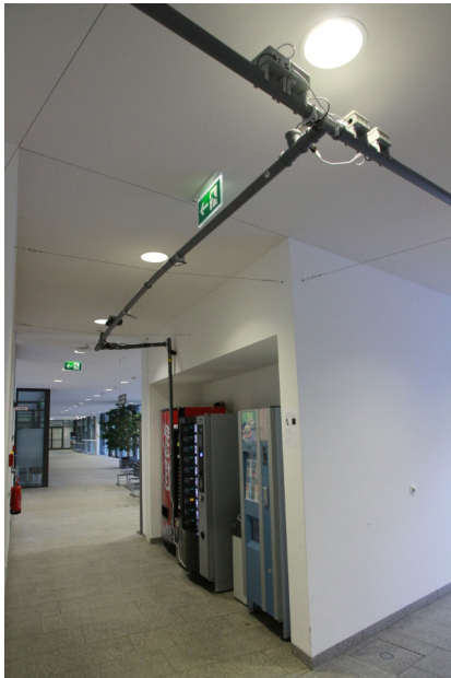
(c) T-crossing: 8 sensors, 23 days, height 2.80m, and area 31m 2
