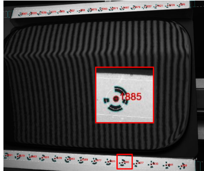
Fig. 6.8: target carrier with fixed markers to define a coordinate \hat{x}_t \hat{y}_t \hat{z}_t that moves together with the object. (courtesy of Simon Hartel)
