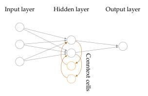
FIGURE 2.8: Illustration of a Elman network [118], a simple Recurrent Neural Network (RNN) using context cells as memory. This context cells are marked in orange.
