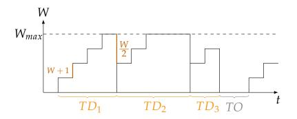
FIGURE 2.1: Illustration of the TCP Reno Congestion Control (CC) [44], with a description of the time until triple duplicate acknowledgments  $(TD_i)$  and the TCP Retransmission Timeout Period  $(T_O)$  due to timeout as well as their impact on the congestion window size (*W*).
