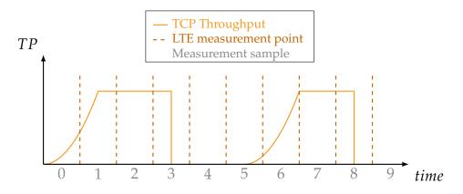
FIGURE 2.2: Schematic diagram of the measurement process, showing the TCP Throughput (TP) as graph over time and the measurement intervals divided by the vertical dashed lines, adopted from pre-published results [52].
