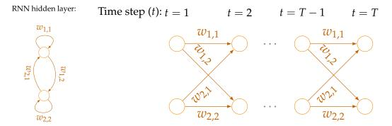
(a) The diagram of a layer with two Recurrent Neural Network (RNN) cells connected to each other and themselves.
