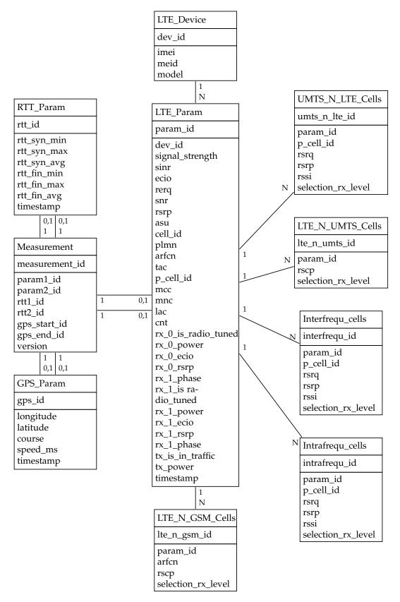
FIGURE 4.16: Database model of the SQLite database used by the measurement tool presented in Figure 4.14, to store the Latency (LA) measurements.
