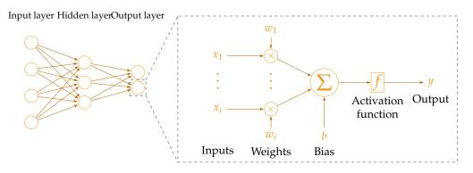
FIGURE 2.6: Illustration of a simple Feedforward Neural Network (FNN) with one hidden layer, four inputs and two outputs. Each circle describes a simple neuron used in feed forward networks. The figure is adopted from prepublished results [77]
