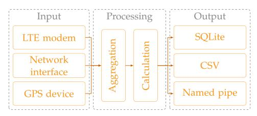
FIGURE 4.1: Structure of the measurement tool, including the input, processing and output modules as presented in pre-published results [52].
