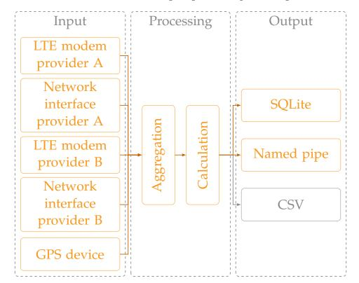
FIGURE 4.14: Structure of the measuring tool, including the input, processing and output modules as presented in pre-published results [52].
