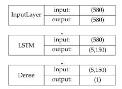
FIGURE 4.9: Structure of the fifth Long Short-Term Memory (LSTM) Recurrent Neural Network (RNN) configuration applied to  $FS_{\Delta y}^{I,e,l}$ . The model contains a layer with Long Short-Term Memory (LSTM) cells as well as a dense layer to output the prediction result.
