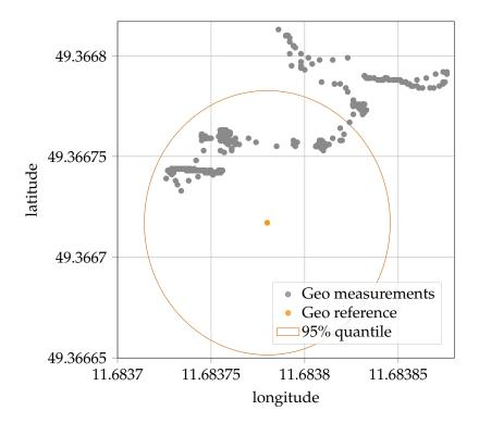
FIGURE 4.2: Visualisation of the GPS accuracy of the built-in Global Navigation Satellite System (GNSS) module, measured on the Geo reference point in Kastl, Bavaria, Germany [194]. Each grid cell has an edge length of approx. 5.5 *m*.
