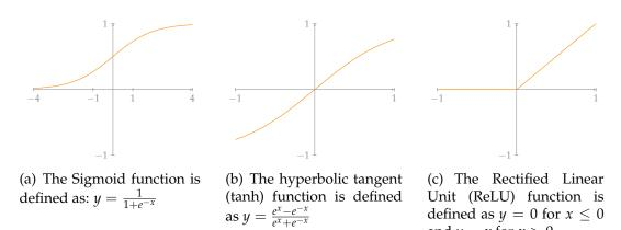
FIGURE 2.7: Commonly used forms of non-linear activation functions [102] included in the neurons of Artificial Neural Networks (ANNs).
