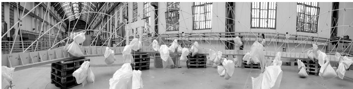
Figure 1-3: Loading test on a hemispheric irregular gridshell of 10 m diameter (Chapter 5)
