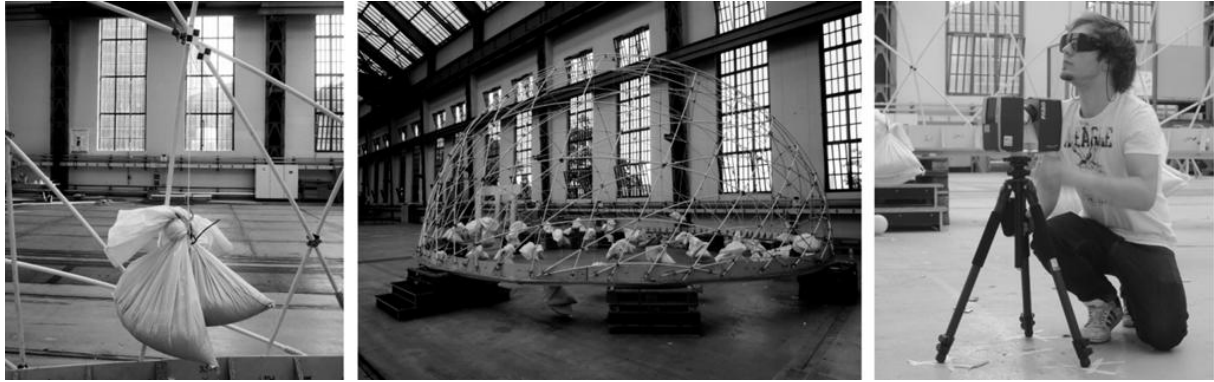
Figure 5-11: Hemispheric gridshell during loading tests and registration of the resulting deformations using a three-dimensional laser scanner
