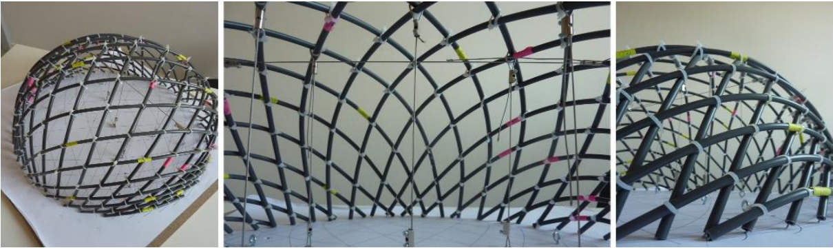
Figure 5-3: Physical 1:10 modelling of the irregular hemisphere
