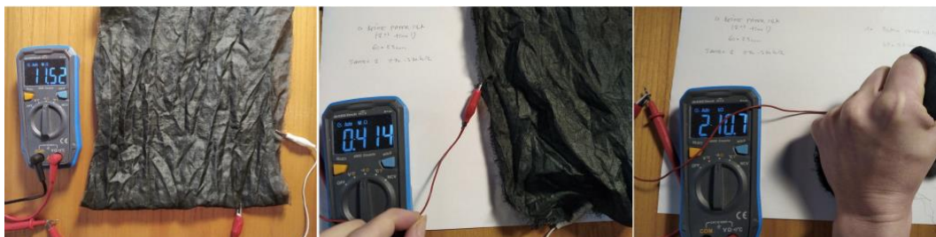
Figure 24: Measuring polymerized paper-silk after first (11.5 M \Omega ) and second processes (from 414 to 210 k \Omega ).
