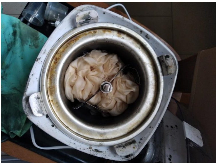
Figure 23: View of beige paper-silk prepared for in-situ polymerization.
