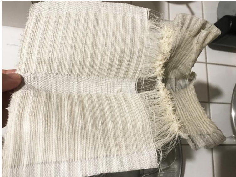
Figure 7: Chirimen sensor matrices before being contact with the finishing bath (left part) and after (right part).
