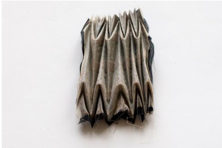
Figure 11: Pleated peacock pressure sensor matrix, 90 x 150 mm (unfolded).
