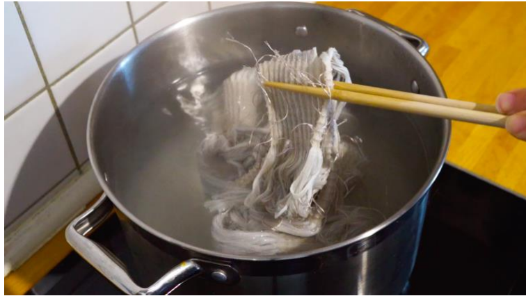
Figure 8: Chirimen sensor matrices being added to the finishing bath.
