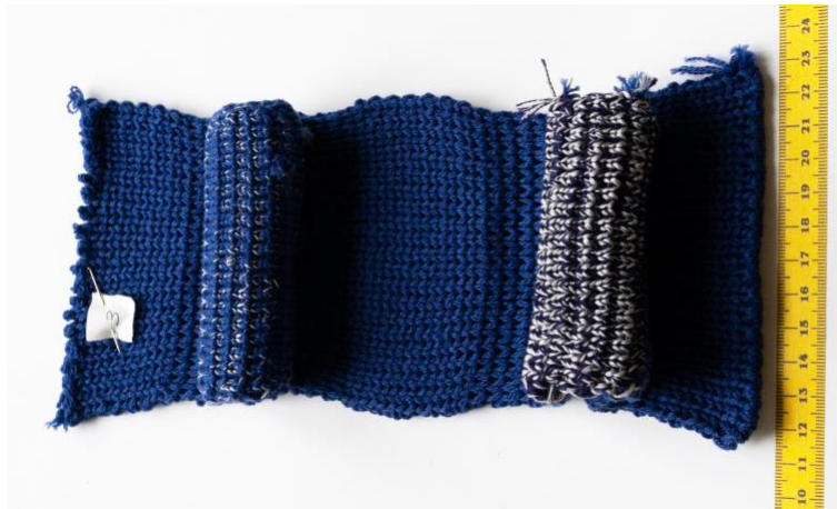
Figure 18: A folded knitted stretch sensor (unit of length: cm).
