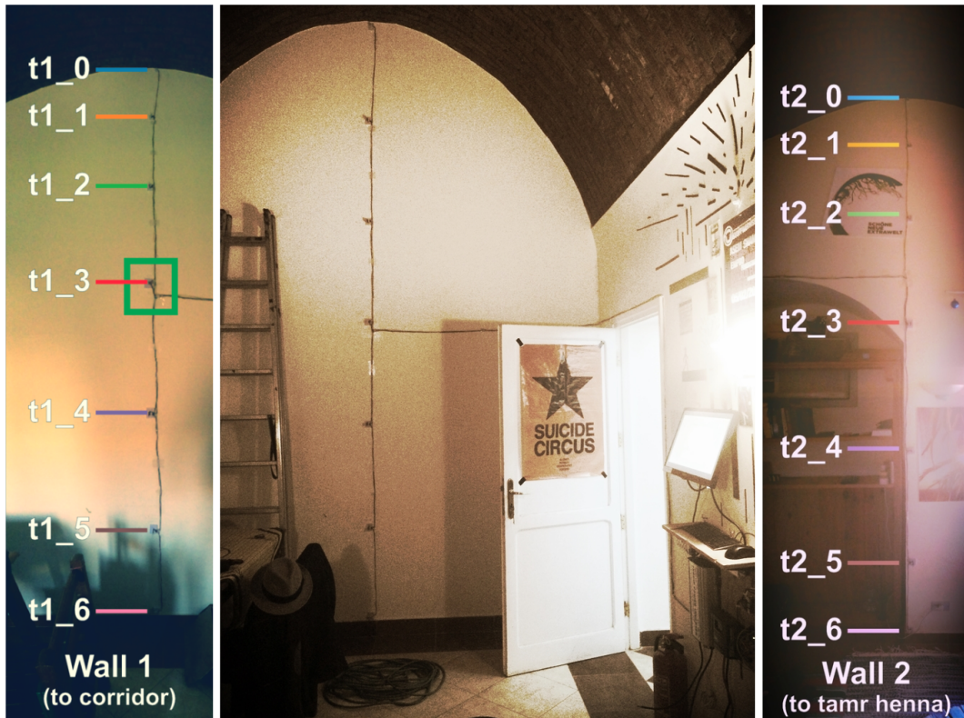
Figure 6.9.: Temperature sensors on both side of the walls and data point names for the living room of the case study apartment H12-214.
