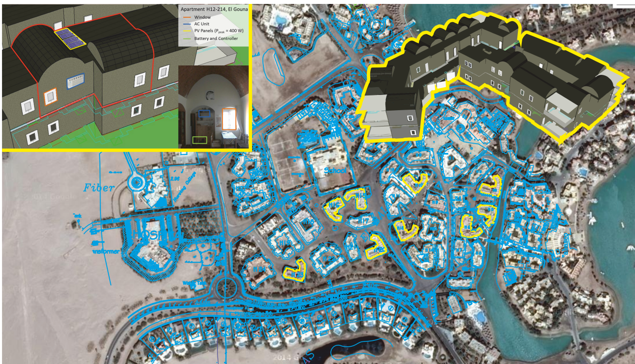
Figure 6.2.: Urban context of simulated apartment in El Gouna, Egypt and IDA-ICE simulation model of the building (top right corner).
