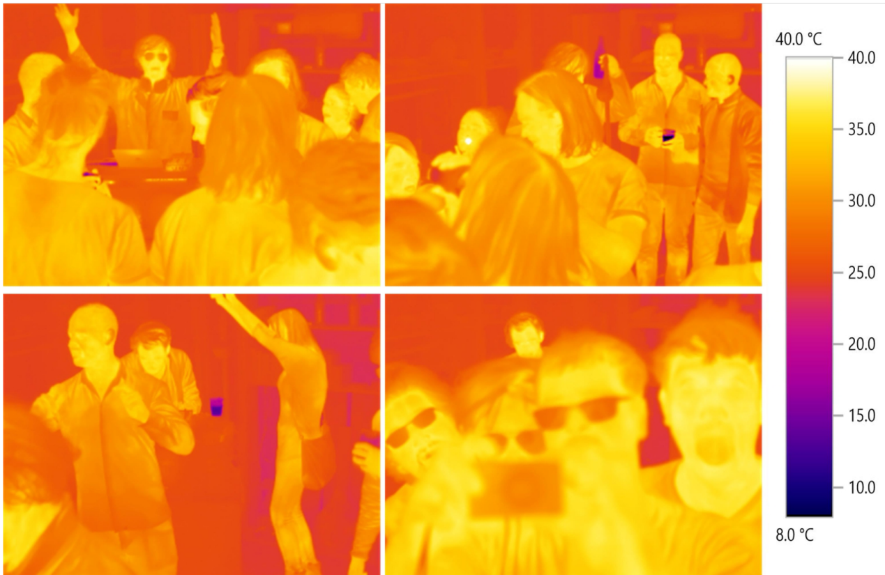
Figure 6.16.: Thermographic pictures during the time from 12:30 to 2 am, showing the variety of different performance states of the internal heat sources.
