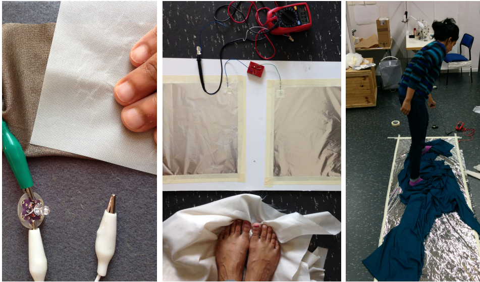
Figure 19. Scaling up the triboelectric circuit and trying out different textile materials and interactions. (Left) Small piece of Teflon baking sheet over conductive fabric swatch. (Centre) Aluminium foil is used to make two conductive tiles connected to a diode bridge and multimeter. (Right) A piece of foil blanket on the floor provides a large conductive floor to explore the electrification process through playful interactions.
