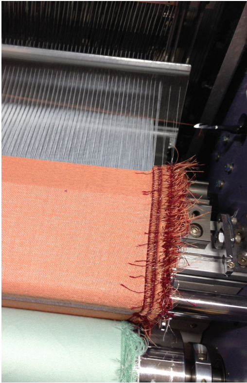
Loom: CCI SAMPLING 16 Shafts (1-16) 40 cm width 12 Colours weft Warp: White Polyester Nm 40/2, 30 thr/cm
