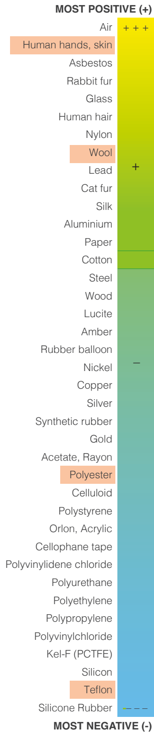
Figure 8. Triboelectric series: materials listed according to their tendency to gain or lose electrons. Figure of the table redrawn from http://eesemi.com/tribo_series.htm
