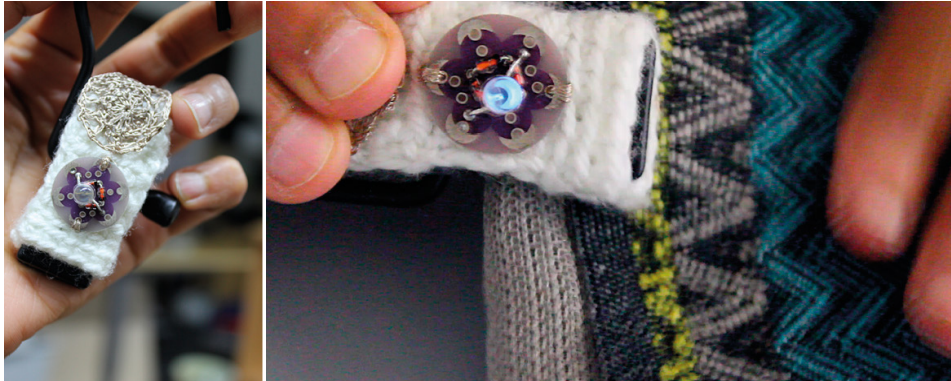
Figure 15. (Left) The clip-on tester. (Right) The tester is clipped to the sample and held with one hand while tapping or rubbing the fabric with the other hand. The LED lights up when enough voltage is generated.
