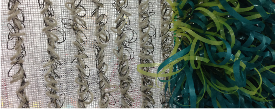
Figure 18. Sample 4a tufted with smaller conductive loops and filled in between with rows of plastic yarn.
