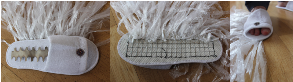
Figure 21. Example of electrostatic material intervention: home slippers that collect the electrostatic charges generated through walking.
