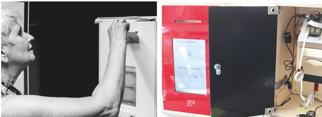
Fig. 71. Hybrid Letterbox: The first prototype (left), and second iteration (right) had different base setups.
