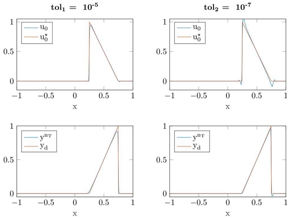
Figure 4: Optimal Control Problem. Optimal control  $u_0^*$  and target  $y_d$ , numerically computed optimal control  $\mathbf{u}_0$  and corresponding state solution  $\mathbf{y}^{nT}$  for tolerances  $tol_1 = 10^{-5}$  (left) and  $tol_2 = 10^{-7}$  (right) using WENO3 with mesh size  $\Delta x = 0.005$ .
