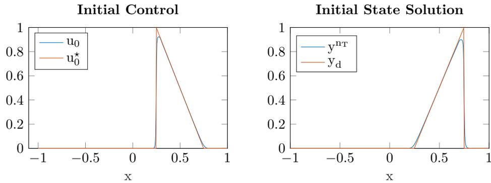
Figure 3: Optimal control problem. Initial control  $\mathbf{u}_0$  and optimal control  $u_0^*$  (left), initial state solution  $\mathbf{y}^{nT}$  at  $T = 0.5$  and target  $y_d$  (right), computed with the WENO3 scheme and mesh size  $\Delta x = 0.005$ .
