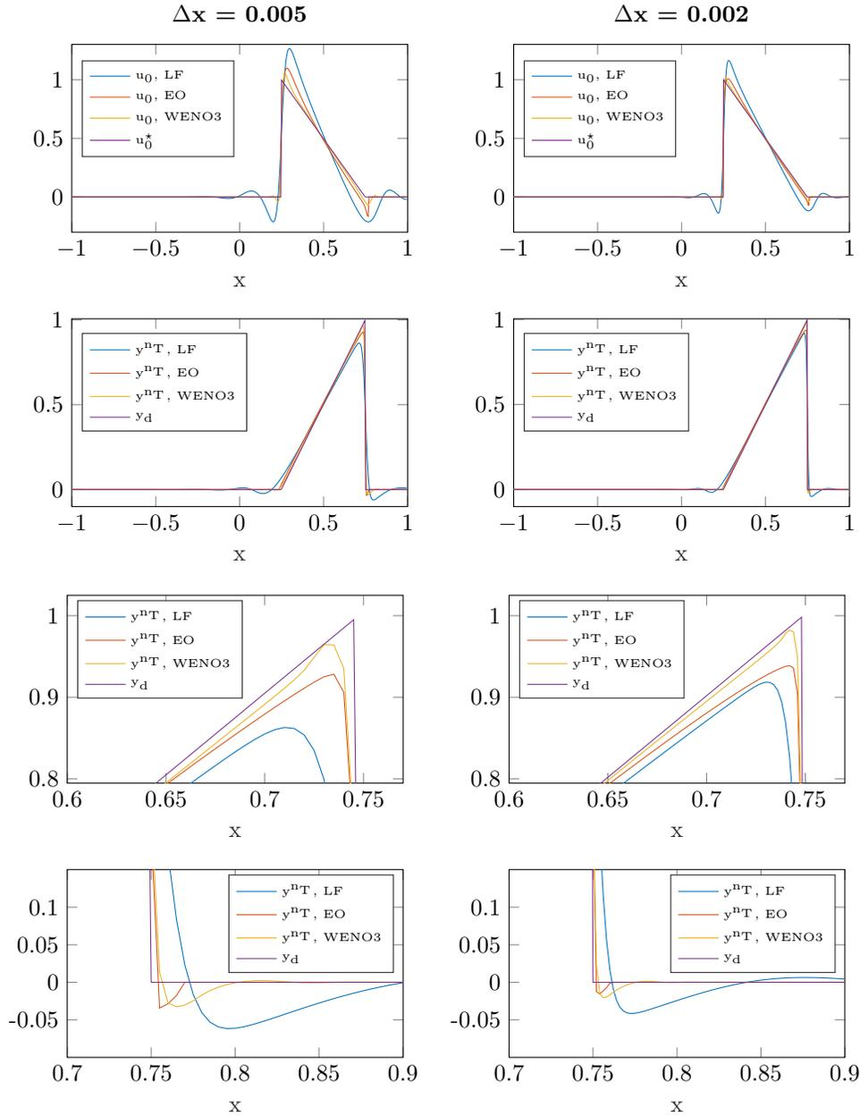
Figure 5: Optimal control problem. Computed optimal control functions  $\mathbf{u}_0$  (top) and corresponding state solution  $\mathbf{y}^{nT}$  (above the middle) with a zoom into the shock region (below the middle, bottom) for 50 iterations of the gradient based optimization algorithm, using LF, EO, and WENO3 scheme with mesh size  $\Delta x = 0.005$  (left) and  $\Delta x = 0.002$  (right).
