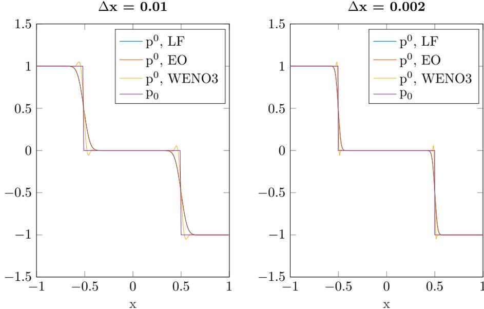
Figure 2: Burgers problem with discontinuous initial and final solution taken from Example 2.1. Numerical approximations  $\mathbf{p}^0$  to the reversible solution  $p_0 := p(0, x)$  given in (11) for the adjoint Lax-Friedrichs (LF), Engquist-Osher (EO) and WENO3 scheme applied with  $\Delta x = 0.01$  (left),  $\Delta x = 0.002$  (right), and  $\Delta t = 0.25 \Delta x$ .
