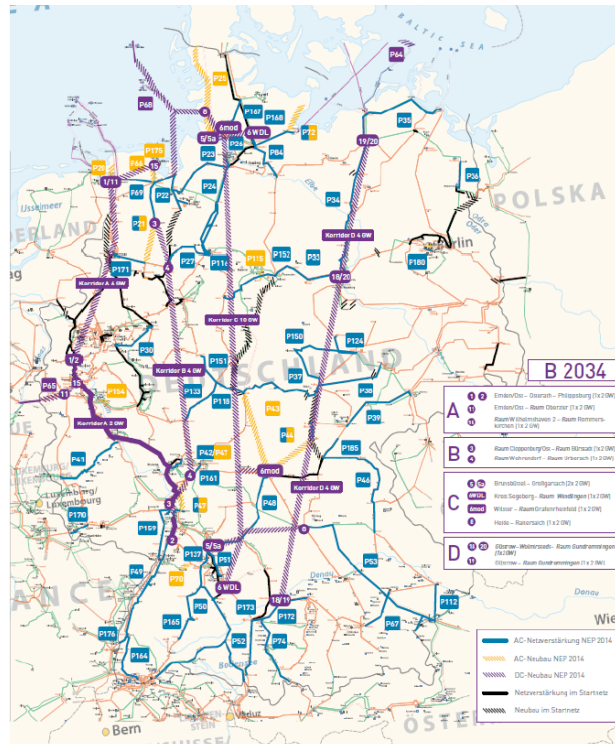
FIGURE 11. Network expansion measures of the NDP 2014, scenario B 2034. Source: German TSOs (2014a).
