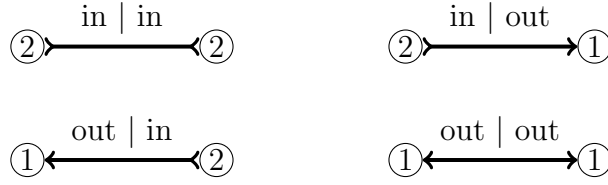
FIGURE 7.1. Number of boundary conditions required for different flow situations. The closed pipe corresponds to two outflow vertices.
