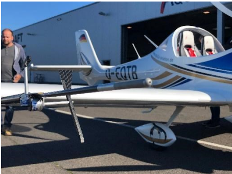
Fig. 8: Air data probe attached to wing
