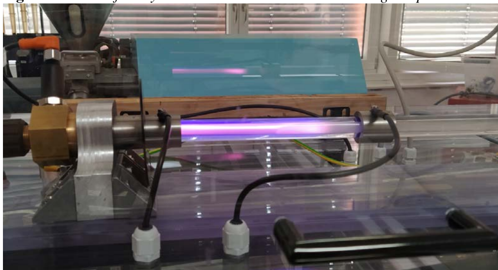
Figure 2. Section of the System with the Plasma Generated during Sample Treatment
