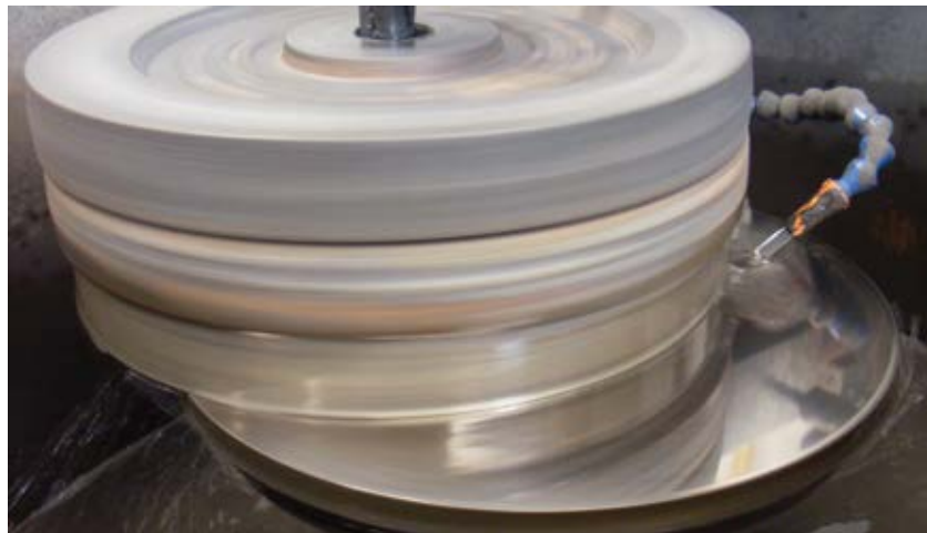
Bound abrasive grinding of a glass plate (top) using an abrasive disc (bottom) and an aqueous cooling lubricant.
