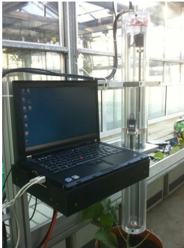
Figure 1: Computer-controlled automatic minirhizotron system.
