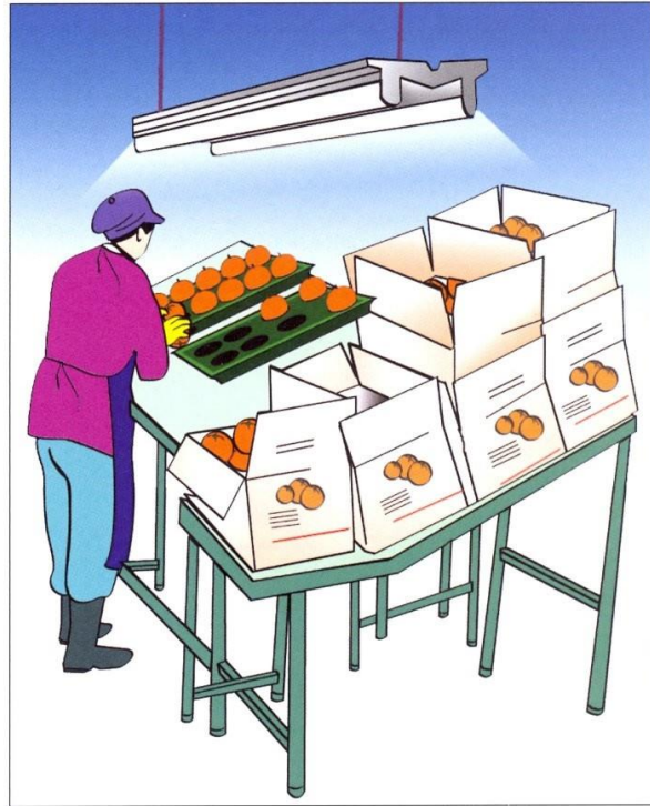
Figure 50b. Make sure that the lights are bright enough without causing shadows or glare.
