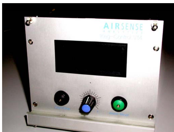
Figure 2-42: Prototype of the electronic nose for the use in biogas plants „biogas nose“
