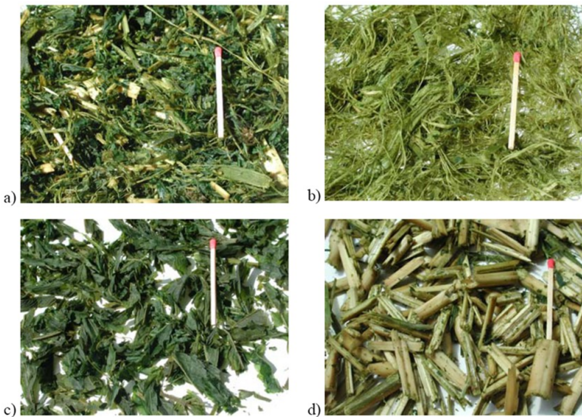
Fig. 5: Manually sorted, chopped hemp: a) chopped material, b) fibres, c) leaves, d) shives (PE-CENKA et al. 2007)
