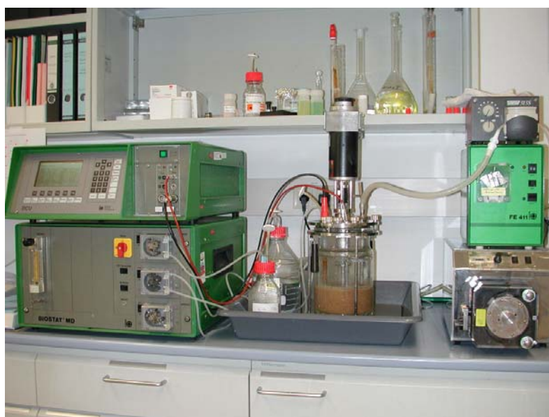
Figure 7: BIOSTAT MD (B. Braun Biotech International GmbH, Germany) equipped with a digital control unit DCU
